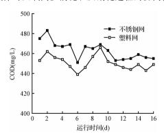
图 6 单一反硝化时出水中 COD 含量变化 Fig. 6 Change of COD content in effluent during single denitrification
