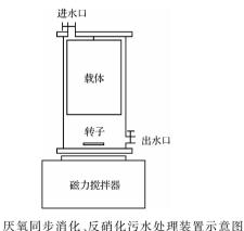
Fig. 1 Schematic diagram of wastewater treatment system for anaerobic simultaneous digestion and denitrification
