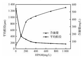
图 1 HPAM 浓度对油含量及油珠平均粒径的影响 Fig. 1 Effect of HPAM density on oil content and oil droplets average particle size
